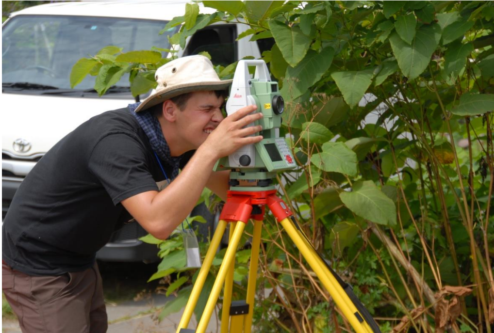
A MacEwan student on archaeological survey crew working the laser Total Station.
