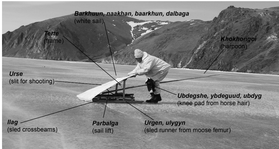
Figure 4. Names of sled parts for ice hunting (photo of V. Khagutov, 2012).
